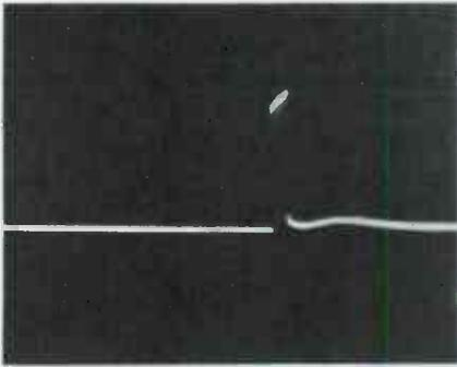
Fig. 6. Expanded vertical sync pulse.
