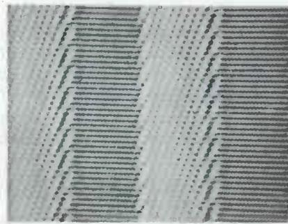
Fig. 12. Fine tuning near sound end, with 4.5-mc carrier off at generator.
