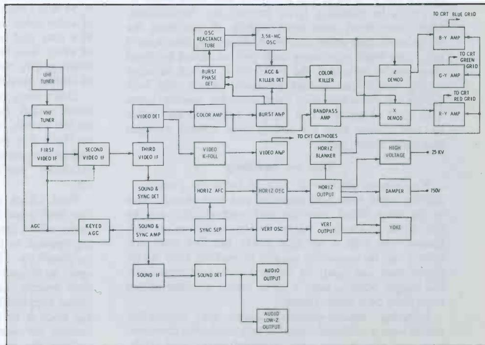
Fig. 1. Stage-by-stage layout of color-TV receivers, showing signal paths.
