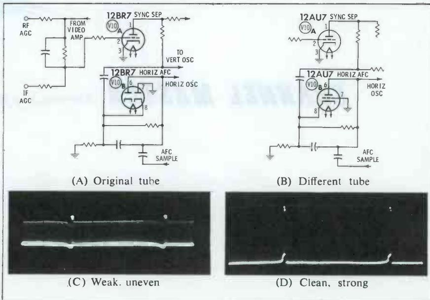
Fig. 5. Circuits and waveforms show improvement brought on by tube change.
