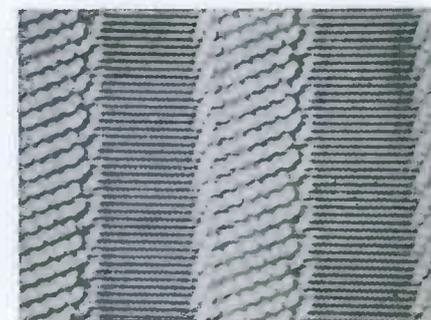
Fig. 7. Effect seen in keyed-rainbow pattern with fine tuning at "sound" end.
