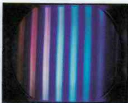
Red content of color picture is smeared and faded; fine-tuning control won't correct trouble. Black-and-white picture shows no evidence of smear or ringing. Color-bar pattern also shows red smear. Other colors are okay, clearing video-IF, chroma-bandpass circuits.
