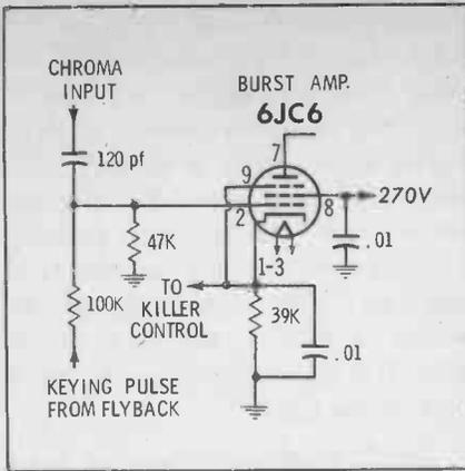
Fig. 8. Burst amp is frame-grid tube.
