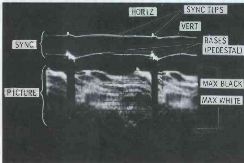
Fig. 1. Makeup of composite video waveform showing relative amplitude of sync.
