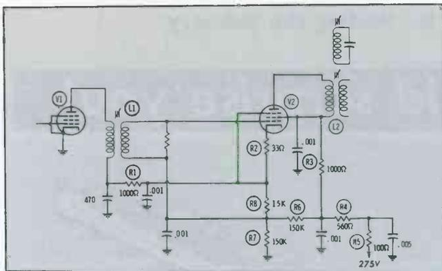
Fig. 2. First video-IF receives B+ from cathode of second.
