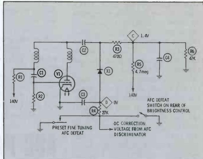
Fig. 8. Divider network holds bias potential on diode X1.
