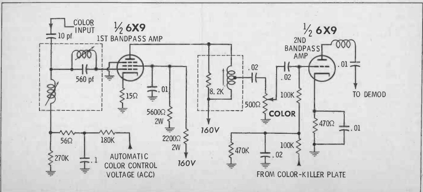
Fig. 3. 6X9 operates in both bandpass amplifier stages in the new Admiral receivers—ACC controls first section.
