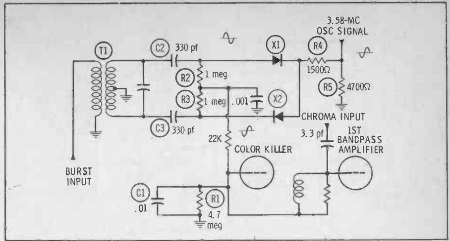
Fig. 4. ACC voltage governs gain of bandpass amplifier in this Philco design.
