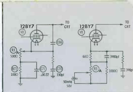
Fig. 10. Changing bias-operated contrast circuit to a variable-degeneration.
