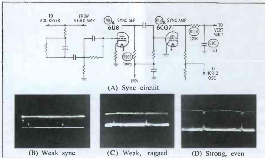
Fig. 9. Modifications in this color-set stage eliminate recurrent sync fault.
