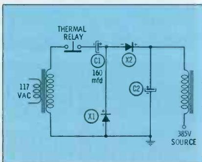
Fig. 1. Doubler circuit, thermal cutout.
