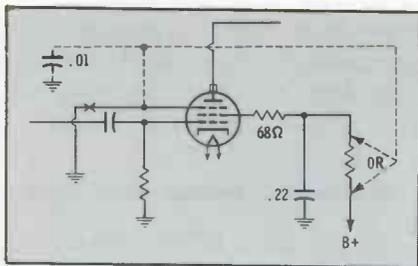
Fig. 4. Change connection of suppressor to eliminate Barkhausen lines.
