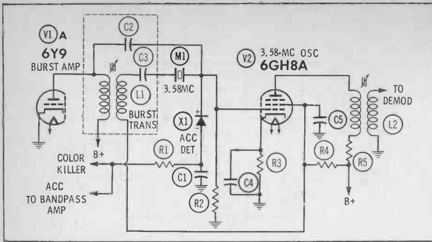
Fig. 6. 3.58-mc oscillator in Admiral G11 chassis operates without burst present.
