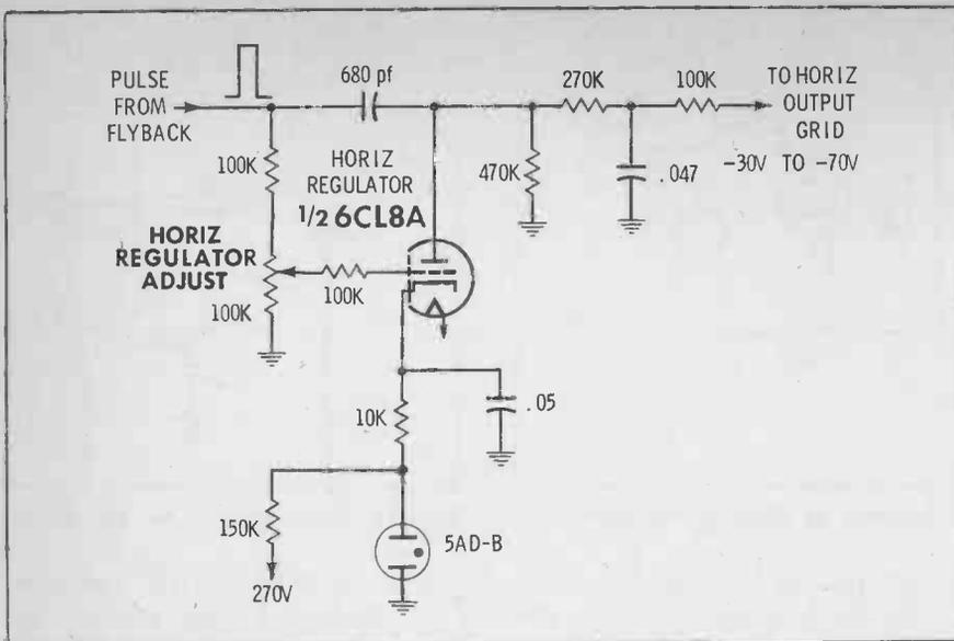
Fig. 15. Sylvania has triode section of a 6CL8A operating as horizontal regulator.
