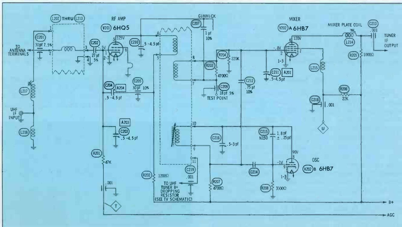
Fig. 2. Alignment adjustments in a typical color-set tuner are identified by "A" numbers.
