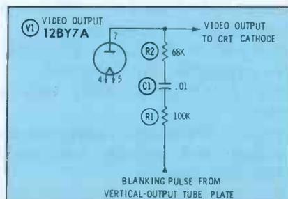
Fig. 5. Video-output tube plate is mixing point for vertical-blanking pulse.
