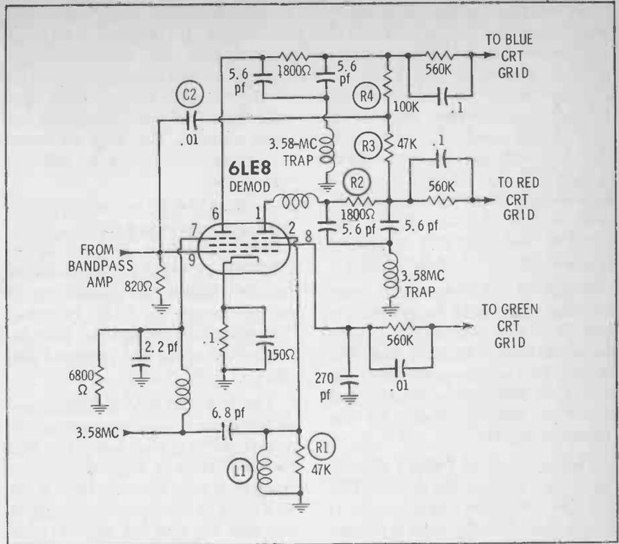
Fig. 9. Single demodulator tube develops difference signals in the Admiral G11.
