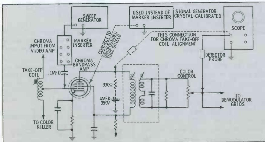
Fig. 5. Necessary test-equipment connections in chroma-bandpass circuit.
