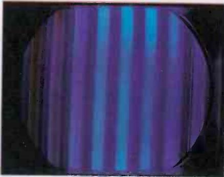
With brightness control at maximum setting, screen still is dim for both color and black-and-white pictures. Bar at far right should be green; instead, is dark blue and barely visible. Absence of a color indicates trouble in chroma, not luminance, circuits.
