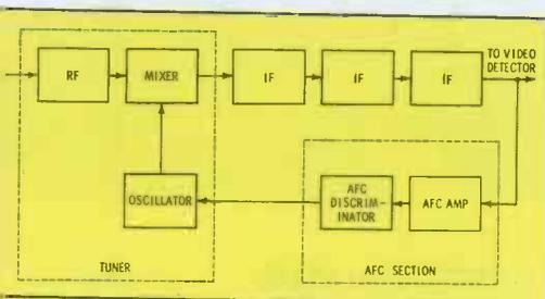
Fig. 1. AFC system is merely feedback loop for correcting oscillator drift.
