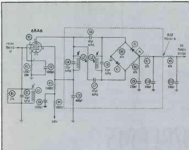
Fig. 7. Schematic of AFC section shows bridge discriminator.
