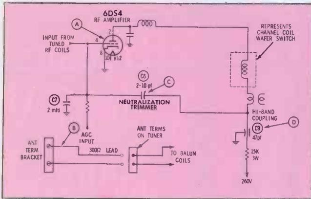
Fig. 3. Oscillation occurs with stage improperly neutralized.
