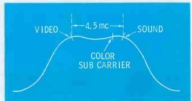
Fig. 1. The VHF-tuner response curve should look like this.
