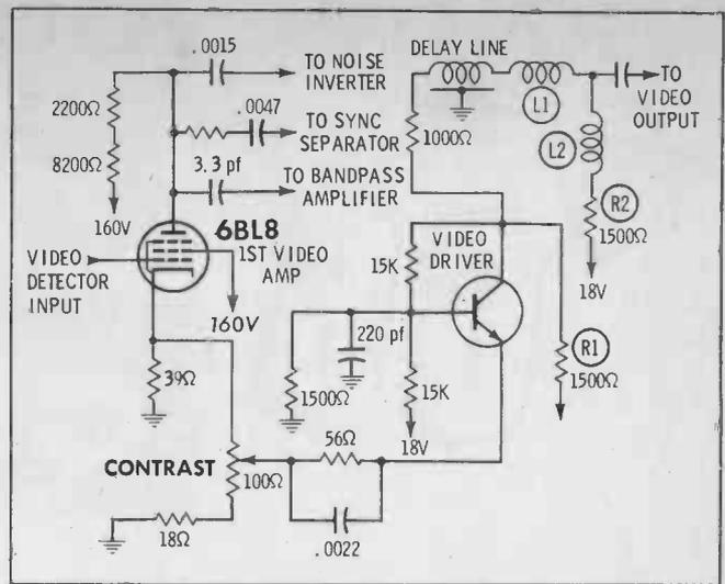
Fig. 2. Transistor serves as video driver in Philco's set.
