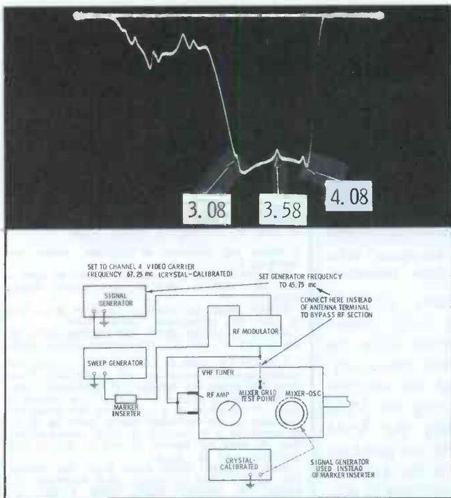
Fig. 8. Setup for video-sweep modulated (VSM) alignment.
