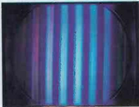
Black-and-white picture is tinted blue. At normal position of tint control, flesh tones are green; with control fully counterclockwise, they are weak magenta. Color-bar pattern proves red output is weak indicating gray-scale misalignment or chroma-output trouble.
