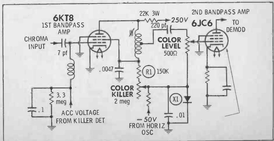
Fig. 5. Zenith derives voltage from horizontal oscillator to cut off bandpass.
