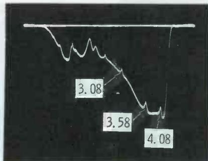
Fig. 10. Misadjusted bandpass take-off coil causes this type distortion.
