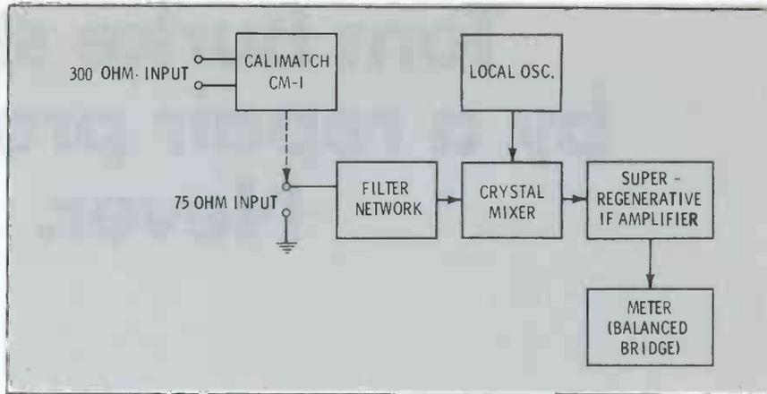
Fig. 4: This instrument may be adapted to either 75- or 300-ohm input.
