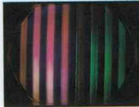
Monochrome picture is deep green or chartreuse. Tint and color controls do change intensity and position of color bars from generator; but blue bars are missing — only green and red visible. Chroma-output or CRT trouble is most likely.
