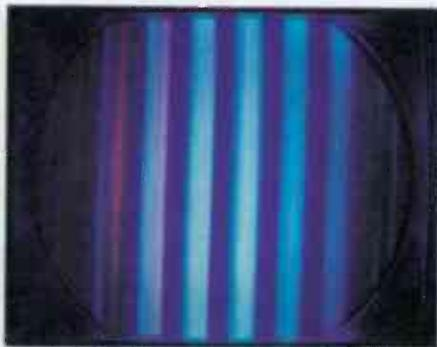
Green content of flesh tones is visible only with tint control fully clockwise; normal setting makes flesh magenta. Monochrome picture turns magenta at low brightness setting. Symptom indicates gray-scale misalignment or chroma-output circuit trouble.
