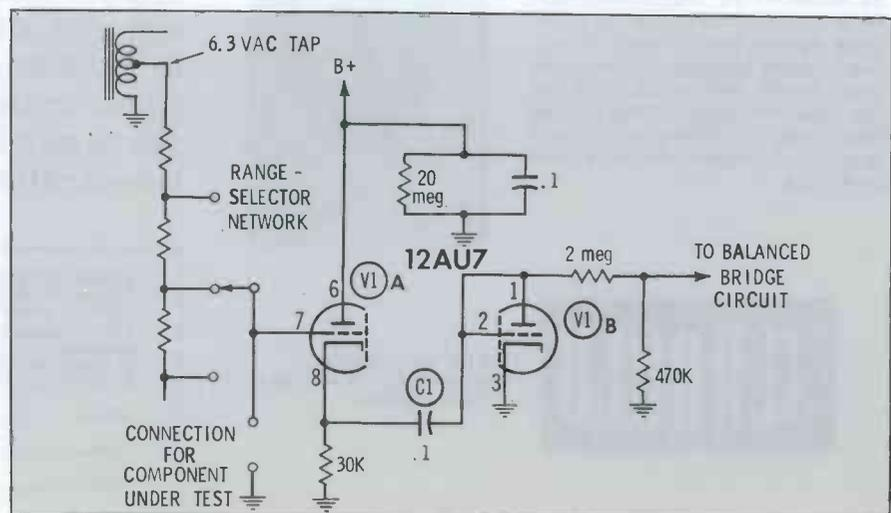
Fig. 2. Circuit arrangement to determine value of capacitors and coils.
