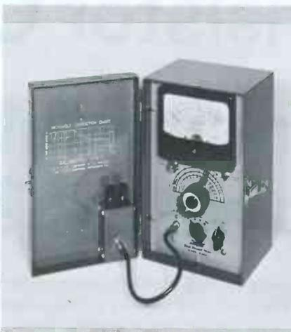
Fig. 3. Portable field-strength meter.
