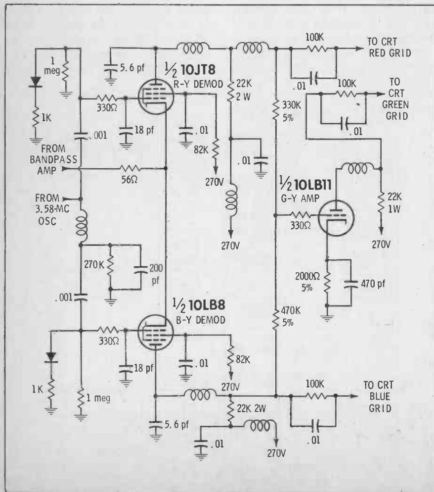
Fig. 11. Sylvania D03 chassis has high-level demodulation and separate G-Y amp.
