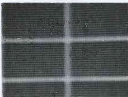
Fig. 4. Dullness in this pattern results from misadjustment of fine-tuning.
