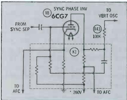
Fig. 7. Reducing series resistor here helps overcome a tendency to jitter.
