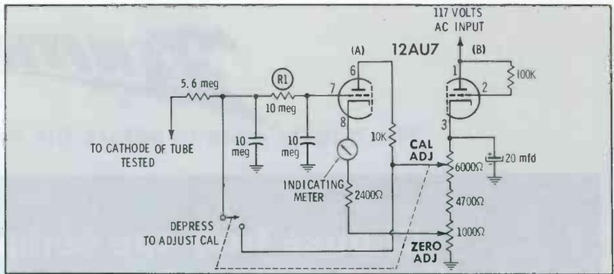
Fig. 7. Vacuum-tube-voltmeter reading will not exceed full scale.
