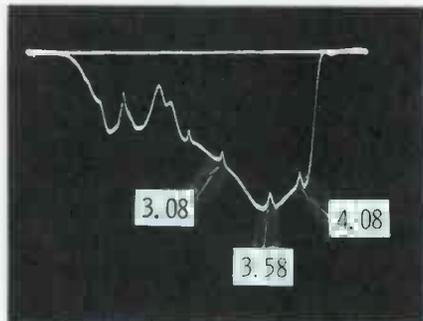
Fig. 9. Video markers should be of nearly equal height on response curve.
