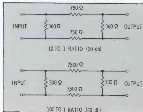
Fig. 5: Pads restrict meter movement.
