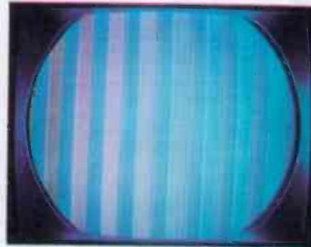
Picture blooms, retrace lines are visible, and brightness is excessive at normal control settings for both black-and-white and color reception. Color is weak, even with color control set for maximum. Washed-out color points to chroma-circuit defect.
