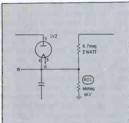
Fig. 3. Special resistor changes value.
