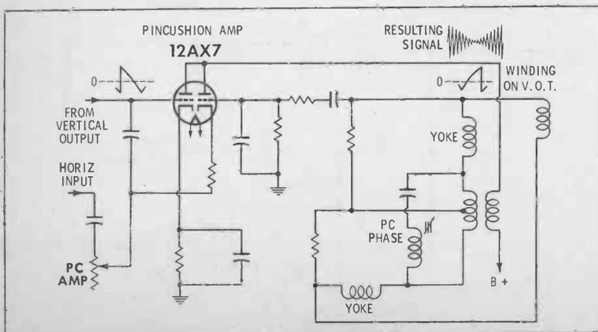
Fig. 16. Magnavox method of obtaining pincushion correction for rectangular tube.
