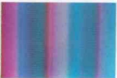
Fig. 11. Misalignment ringing that can also be caused by incorrect fine tuning.
