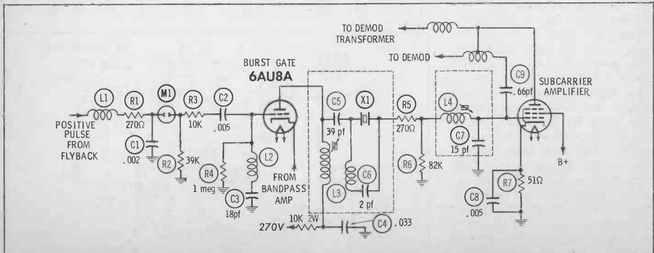
Fig. 7. General Electric's CB chassis uses ringing circuit and a subcarrier amplifier to develop 3.58-mc signal.
