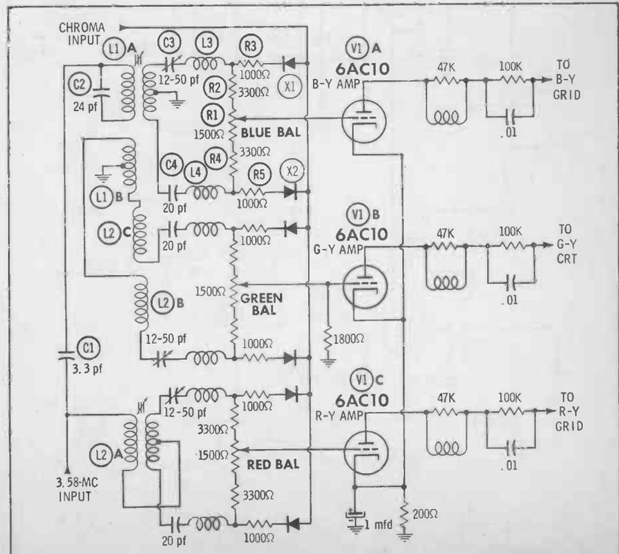
Fig. 10. Demodulator tube(s) is replaced by diodes in new General Electric receiver.
