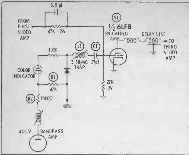
Fig. 1. Color indicator light is controlled by bandpass amp.
