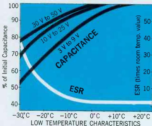
The result: life, reliability, and temperature stability are far superior to cardboard case capacitors and other plastic-case types. Consistently better than imported types. And even better than many metal case tubular capacitors which cost one-third more! Look at the temperature stability test chart, for instance. This is excellent performance for a low-cost miniature electrolytic. So good, in fact, that we have now rated the MTA for  $-30^{\circ}\text{C}$  to  $+85^{\circ}\text{C}$ .
