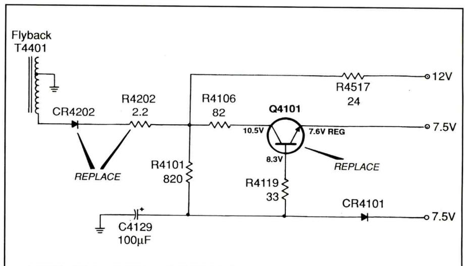
**Figure 8.** Check CR4704, Q4101, and Q4702 in the 7.5V source if the chassis is dead.
