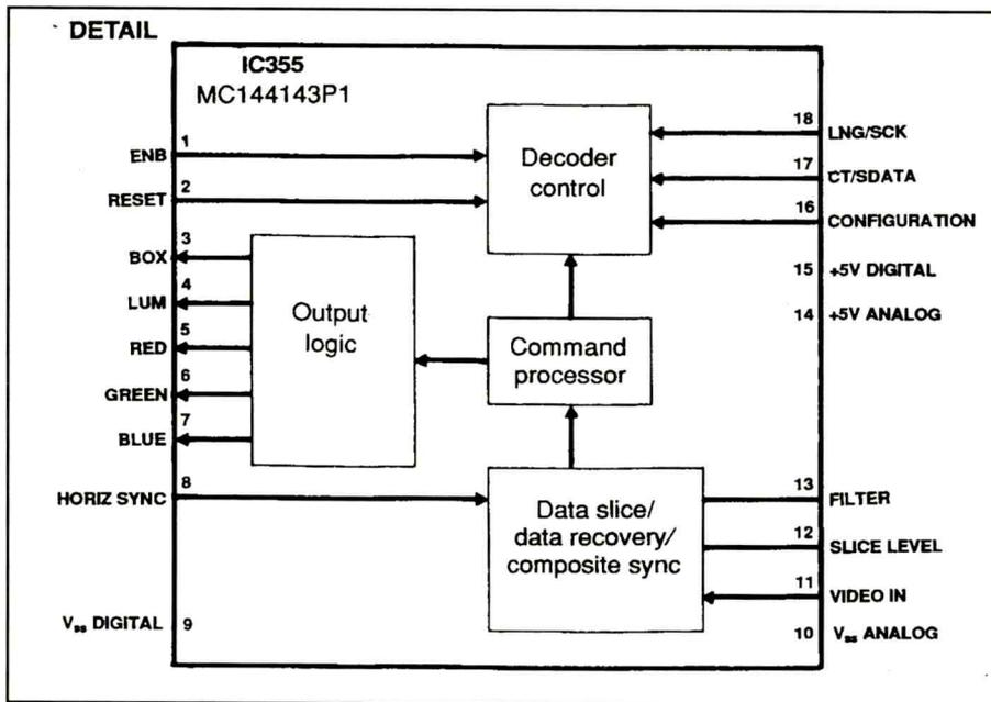
Figure 1b. The internal block diagram of the decoder IC will help you to understand how it functions.
