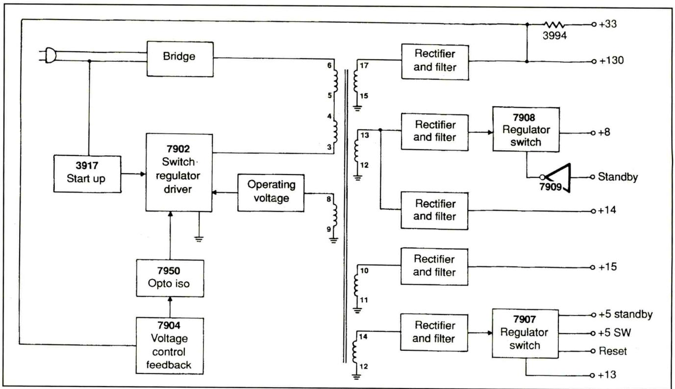
**Figure 1.** This block diagram of the D7 chassis breaks down the circuit down into easily conceptualized units.
