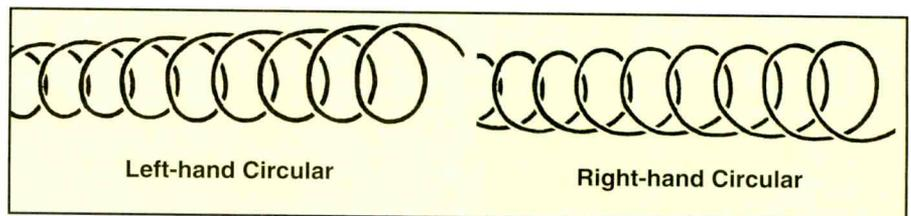
**Figure 4.** Helical antenna design operates on the principle of circular polarization as shown here, rather than the horizontal or vertical polarization found with other antenna designs.
