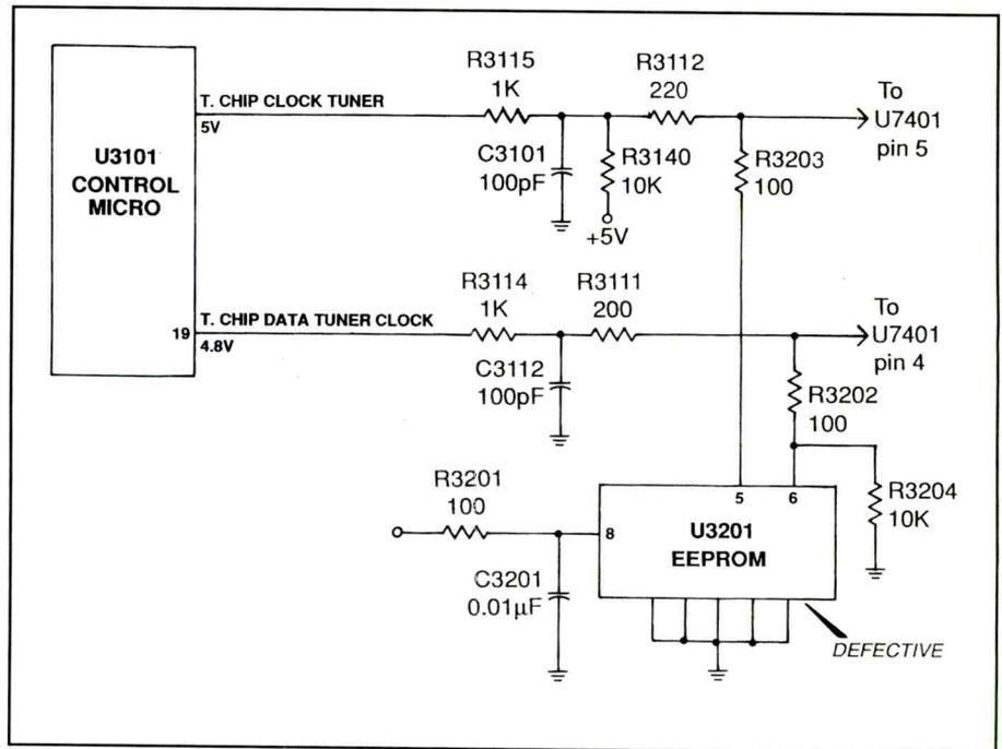
**Figure 2.** A defective EEPROM can cause many different service symptoms in the RCA CTC177 and CTC187 chassis.
