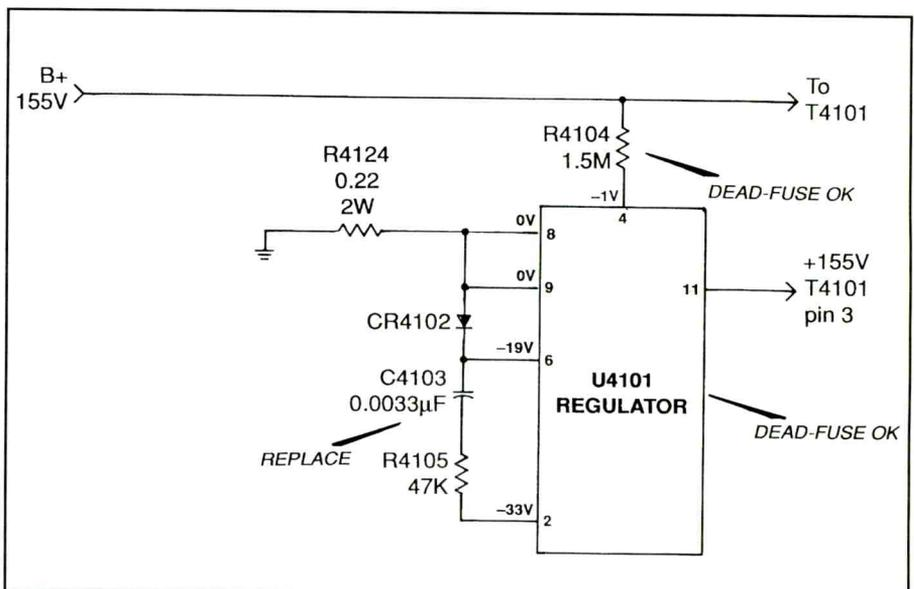
**Figure 3.** A dead CTC187 chassis with normal fuse might be caused by a component around the U4101 regulator IC.
