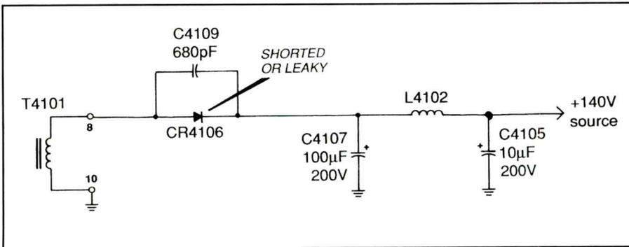
Figure 5. Check CR4106 in the +140V source and Q4105 in the +5V standby source when the problem is a dead chassis.
