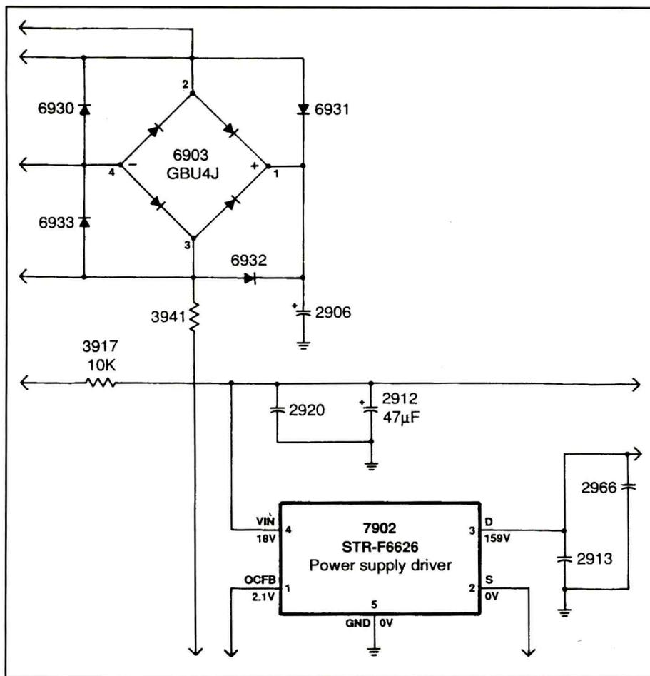
Figure 2. A partial schematic of the primary side of the D7 power supply.
