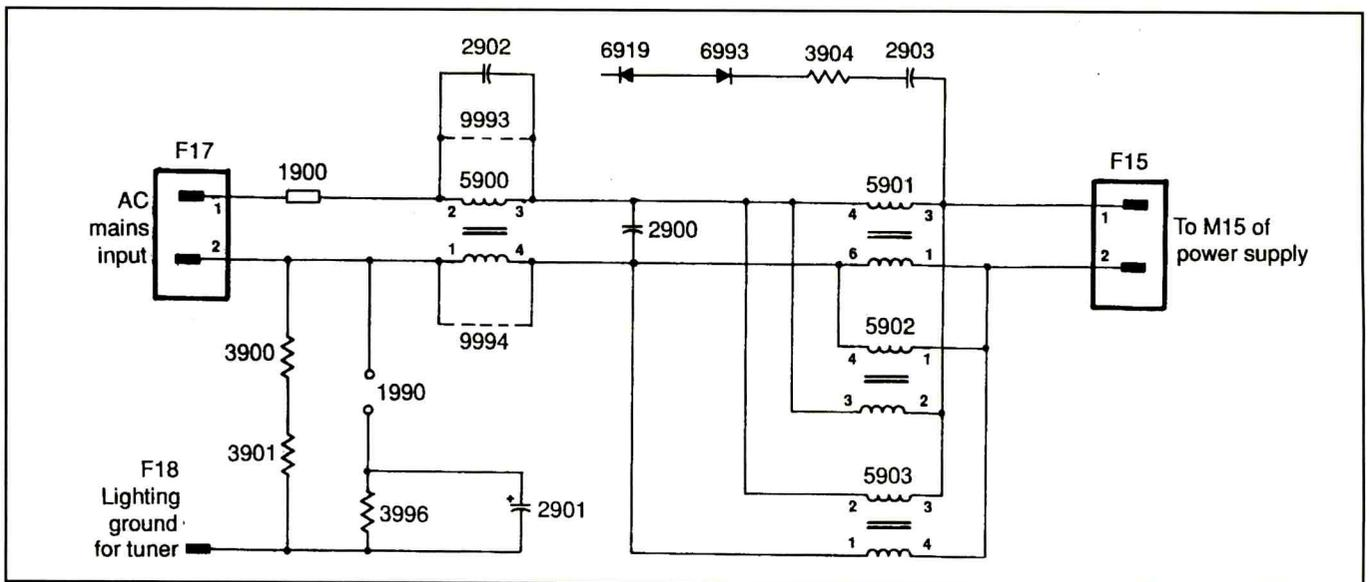
**Figure 3.** In this set, ac is input through what the engineers call a "mains filter," which is a group of components on a separate circuit board consisting of an ac cord, a fuse, capacitors, and chokes.
