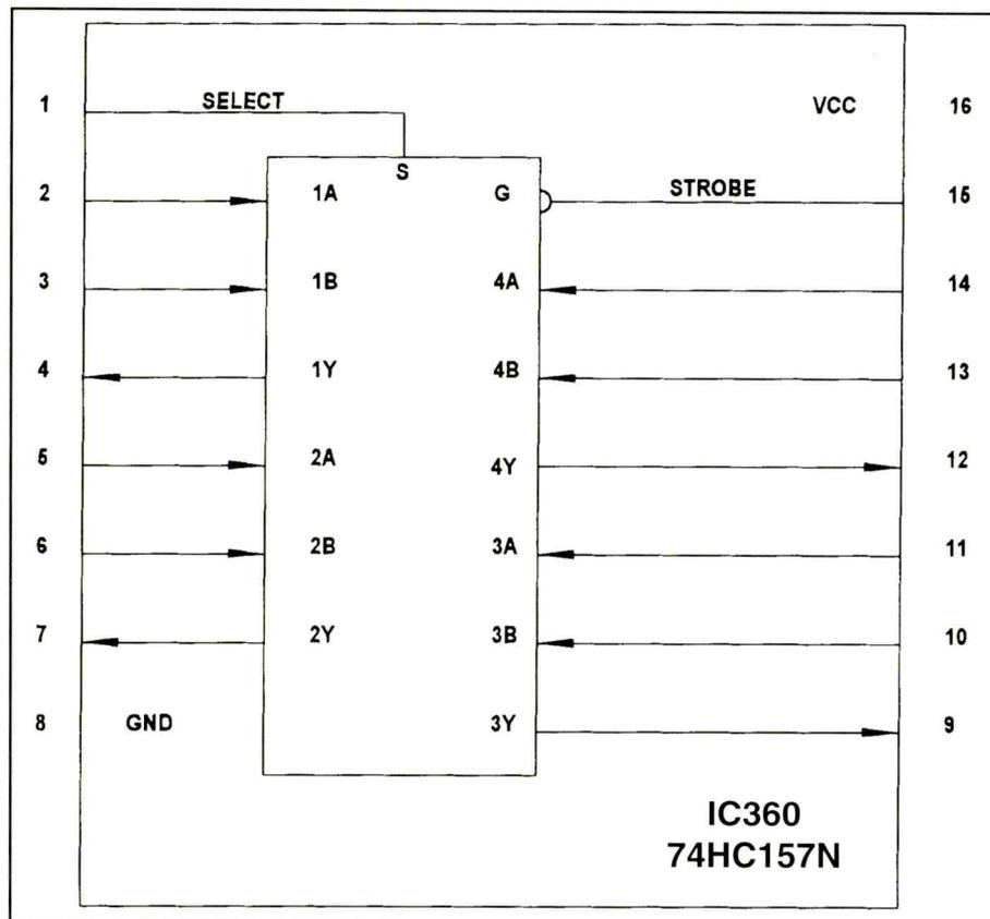
Figure 2. The internal diagram of the quad two-input multiplexer shows that it is essentially four A/B switches.
