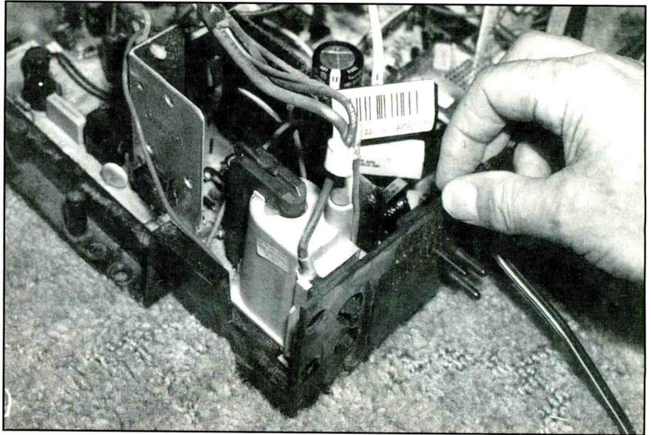
**Figure 7.** Bad soldered connections on the flyback terminals can cause intermittent raster and picture, and sometimes, when arcing, can open the power line fuse.
