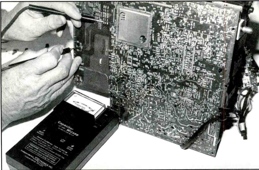
Figure 4. Check for open or soldered trace line in the TV chassis with the ESR meter.
