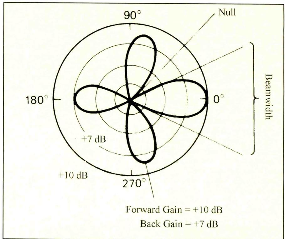
Figure 1. Antennas have characteristic transmission/reception patterns, as shown in this antenna pattern drawing.
