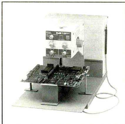
The system features multiple modes of operation, adjustable temperature and airflow, as well as a timer for repeatable operations. Using the integral hot gas jet, the unit can be configured to trace the land pattern of QFPs, SOICs, and
