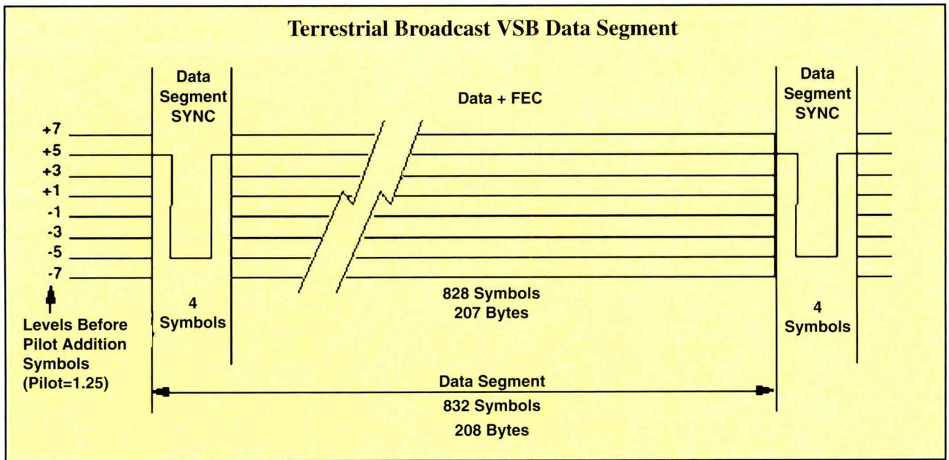
**Figure 2.** The digital television transmission standard takes advantage of the 8-Vestigial Sideband (8-VSB) modulation format and the MPEG-2 (Moving Picture Experts Group) compression/packetization format. The digital transmission standard allows the conversion of high definition studio video into the form used for over-the-air transmission.
