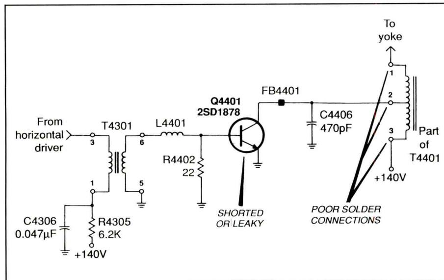
Figure 6. Resolder pins 1, 2, 3, and 10 of flyback (T4401) if the chassis is dead and you hear a whining noise.
