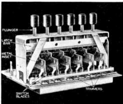
FIG. 6A. Sprague electrical automatic tuning unit with built-in trimmer condensers. The switch blades in the foreground are normally held apart by the strip of insulating material mounted on each plunger; when a button is pressed, the metal inset moves down between the blades, shorting them and closing the circuit to one set of trimmer condensers.
