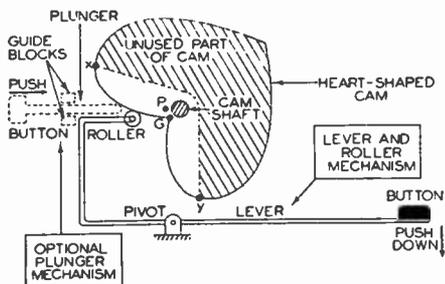
FIG. 3. Operating principles of direct push types of mechanical automatic tuning systems employing a cam with either a lever and roller or a plunger. Pressure on the button in the direction indicated by the heavy arrow serves to rotate the gang tuning condenser (geared to the cam shaft) to the correct setting for the station assigned to that button.
