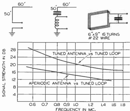
Fig. 1. Signal strength of tuned and untuned antenna compared with a tuned loop.
