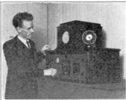
Philo T. Farnsworth, young San Francisco inventor and experimenter, shown with his improved Televisor, constructed in the Crocker laboratories. The white circle is the image screen for reception, the microphone being used for talking sequences.
