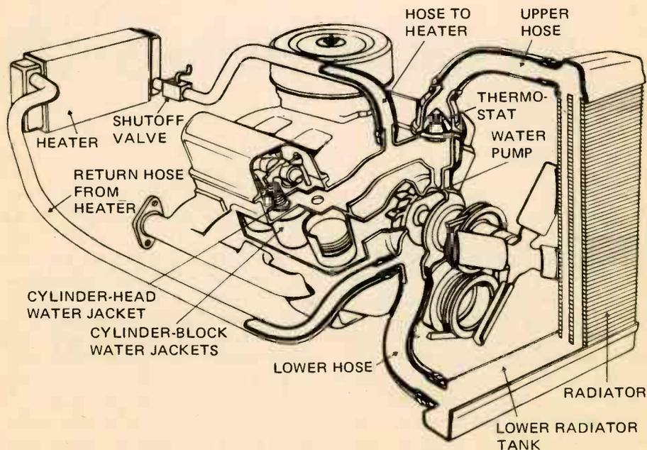
FIGURE 1. A CUTAWAY VIEW OF THE COOLING SYSTEM OF A V-8 ENGINE SHOWING HOSES THAT SHOULD BE CHECKED.
