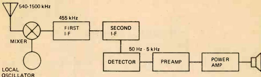
FIGURE 1. SIMPLIFIED BLOCK DIAGRAM OF A TYPICAL AM RECEIVER.
