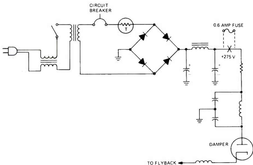
FIGURE 1. POWER SUPPLY AND DAMPER IN PHILCO 21ST90.
