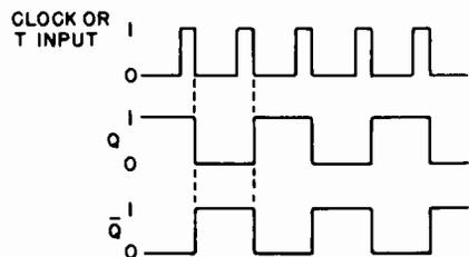
Fig. 8. Waveforms illustrating the toggling of a JK flip-flop.
