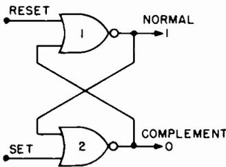
Fig. 2. A NOR gate flip-flop.
