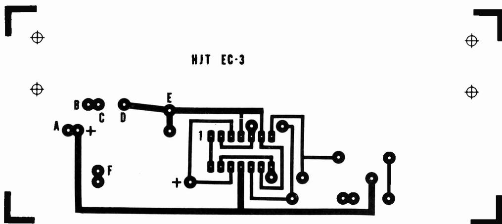
Fig. 2. A printed circuit etching guide.
