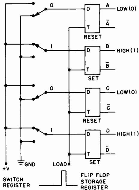
Fig. 5. A switch register and a D flip-flop register storing the binary number 1010.
