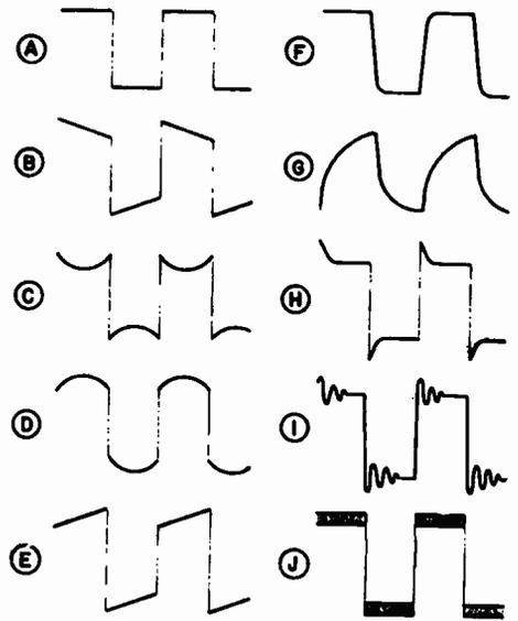
Fig. 6. Typical waveforms. (A) perfect response, (B) low-frequency phase shift — leading (bass cut), (C) loss at fundamental frequency, (D) boost at fundamental frequency, (E) low-frequency phase shift — lagging (bass boost), (F) moderate loss of highs, (G) severe loss of highs, (H) excessive highs, (I) ringing due to instability, (J) thickening of trace due to hum pickup or oscillation.
