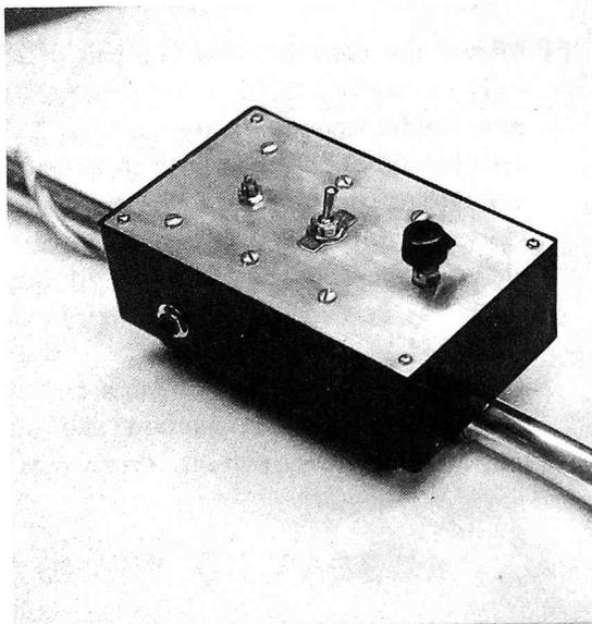
the exploring stem in accordance with Figs. 5 and 6. Route the cable up the exploring stem by first drilling a 1/4" hole in the end of the box nearest the search coil, then running the cable through the hole (Fig. 3) and attaching the cable to the chassis cover (Figs. 2 and 3). You could drill a larger hole and use a rubber grommet. This would keep the cable from sliding in the hole.
