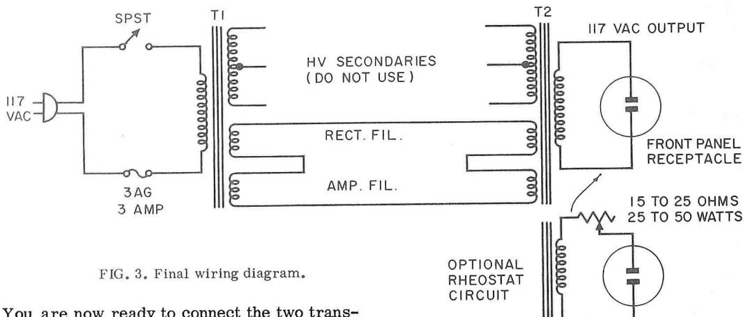
FIG. 3. Final wiring diagram.
