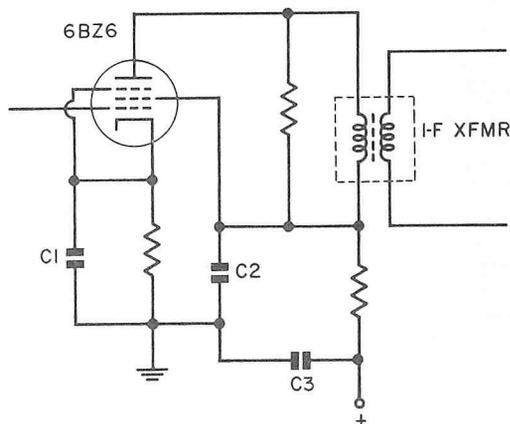
FIG. 2. Bypassing a TV I-F amplifier.
