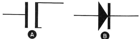
FIG. 4. The thermionic diode, A; the solid state diode schematic symbol. Special-purpose diodes are variations of the solid state symbol.
