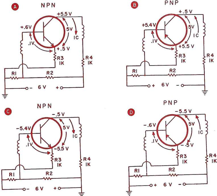
FIG. 1. Basic NPN and PNP transistor circuits. Either the positive or the negative side of the supply voltage may be grounded, as shown above. The voltages between the elements and the chassis depend upon the type of transistor and upon which side of the supply is grounded.
