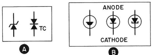
FIG. 9. Zener symbols, A. TC means temperature-compensated zener; most commonly used tunnel diode symbols, B.
