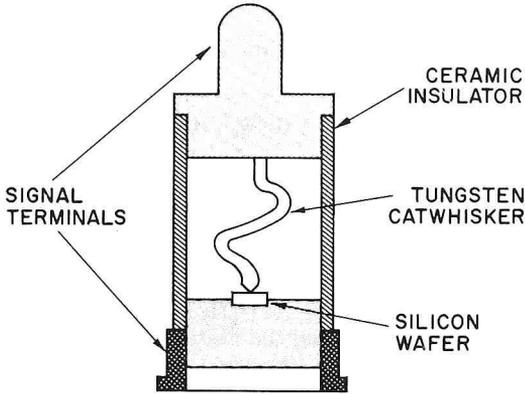
FIG. 2. Cross section of a microwave mixer crystal diode. Note cat whisker similar to old cat whisker receiver crystal.
