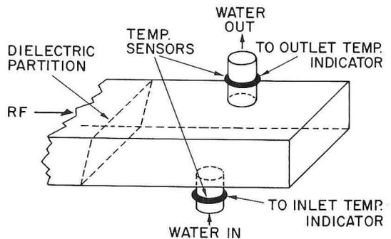
FIG. 4. Section of waveguide housing a water load. Water fills area between partition and end of guide.
