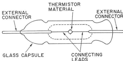
FIG. 1. The glass encapsulated thermistor showing how bead is suspended between leads.
