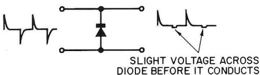
FIG. 7. The diode conducts when the voltage goes negative, removing this half of waveform.
