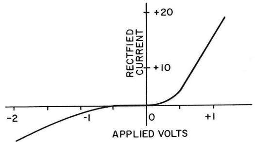
FIG. 8. Curve showing nonlinear characteristic which permits the diode to mix frequencies.
