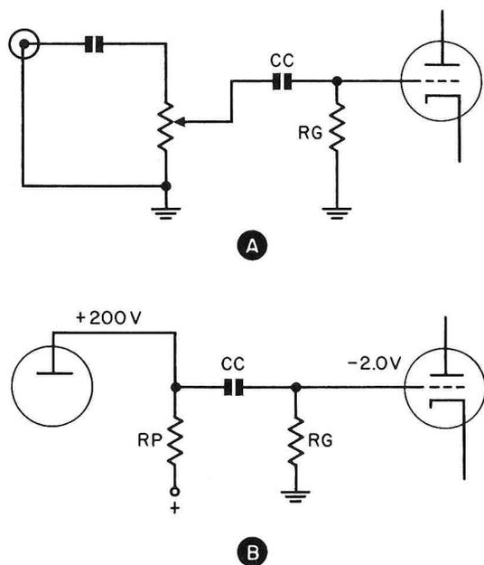
FIG. 3. The coupling capacitor. A, coupling only; B, coupling and blocking.
