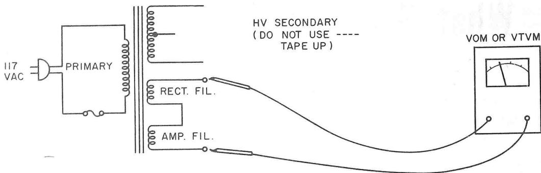
FIG. 2. Connect filament secondaries in series; meter shows if they add or buck.
