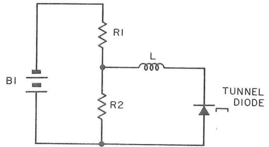
FIG. 2. Schematic showing how a tunnel diode may be used in a simple sine wave oscillator circuit.
