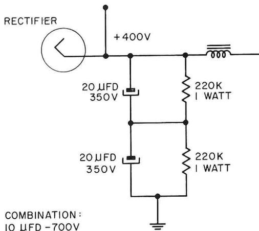
FIG. 5. Series capacitors for higher voltage rating.
