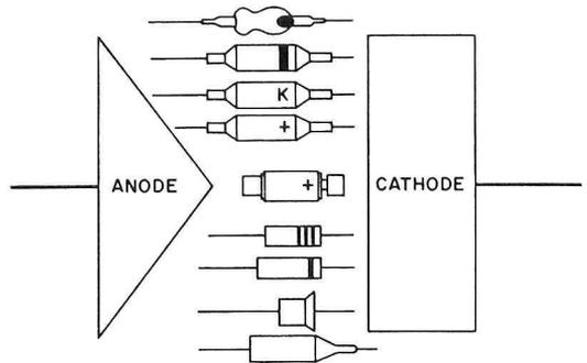
FIG. 3. Diodes showing different construction methods and method of identifying the cathode by various marking methods. The cathode is usually marked. The (+) means the side that a positive voltage would be measured.
