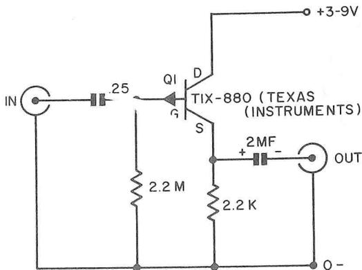
FIG. 4. Circuit showing FET transistor used as an impedance-matching device.
