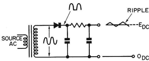
FIG. 5. A familiar half-wave rectifier with waveforms depicting the pulsating voltage and the DC rendered by filtering (plus ripple.)
