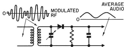
FIG. 6. Diode detector removes carrier and leaves modulation rate.
