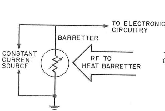
FIG. 7. Barretter circuit with syncogram showing what produces the voltage ramp from the rf pulse.
