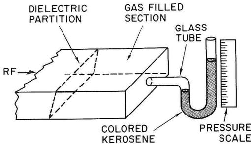
FIG. 5. Gas load showing manometer with scale. Expanding gas moves colored kerosene.
