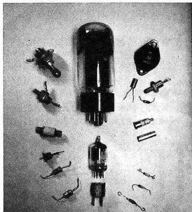
FIG. 1. Types of diodes. Thermionic (center), selenium (bottom). Left side shows display of silicon power rectifiers; at right (top to bottom) are zener, microwave, germanium and silicon signal diodes.
