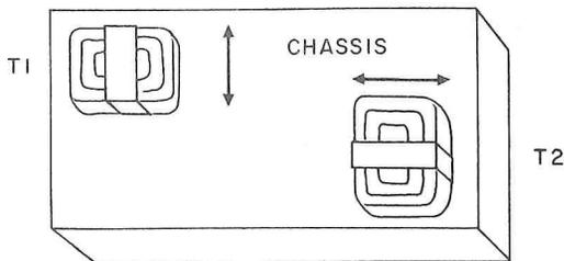
FIG. 4. Place transformer laminations at right angles to each other and as far apart as possible.
