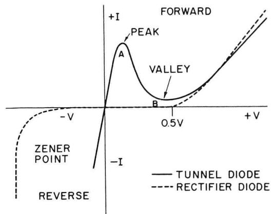
FIG. 1. Voltage-current characteristics of both a tunnel diode and conventional P-N silicon rectifier diode.
