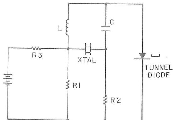
FIG. 3. Use of a tunnel diode as a 100 kc crystal oscillator.
