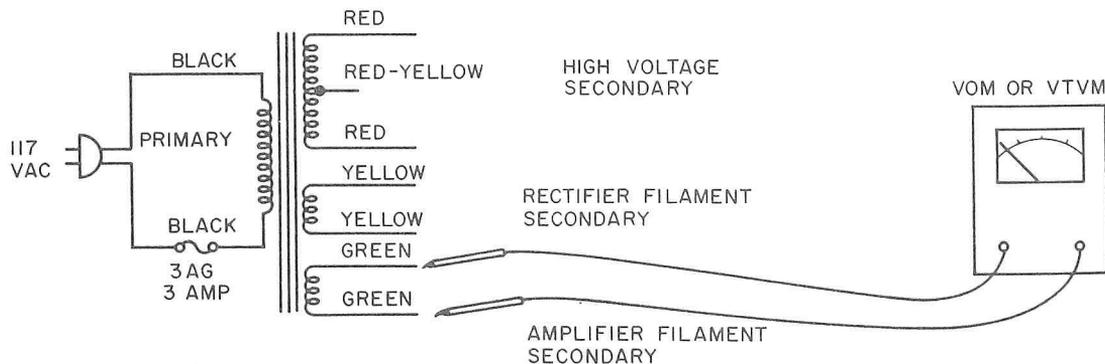
FIG. 1. Measure secondary voltages.
