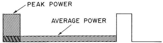
FIG. 3 Pulsed energy. The area under the pulse equals the peak power. The shaded area from one pulse to the other is average power. The ratio is exaggerated for illustrative purposes.
