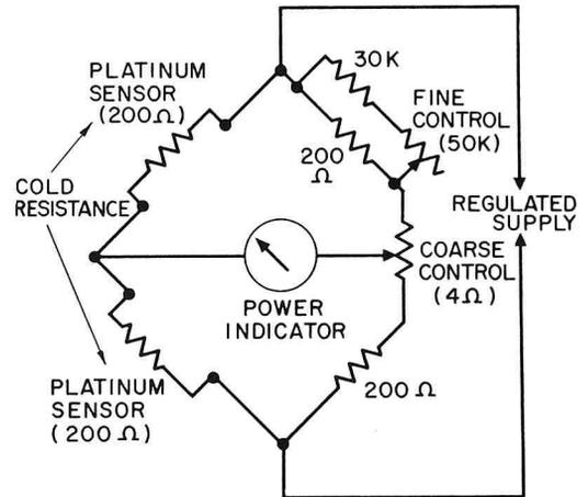
FIG. 6. Johnson meter bridge network. One sensor is on waveguide wall; the other is on constantan section.
