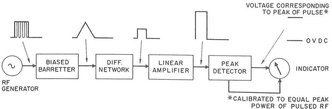
FIG. 8. Block diagram of peak power meter with waveforms. As the peak power varies, the voltage pulse varies proportionally.
