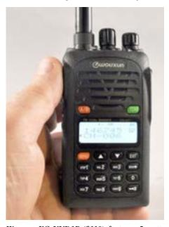
Wouxon KG-UVD1P (\$110) features 5 watts VHF, 4 watts UHF, Li-ion battery, intelligent drop-in charger, flexible SMA-J (female) antenna and belt clip.
