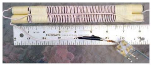
A "Helper Loop" can be easily built with ferrite rods, some wire, and a variable capacitor. (Photo courtesy of John Stoll)
