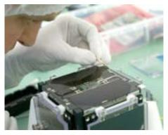
Howard Long G6LVB puts the finishing touches on the flight model FUNcube-1 satellite. (Courtesy: AMSAT-UK)
