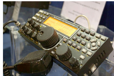
The Elecraft K3/0 Mini is a slim-line faceplate that, when used with the RemoteRig 1258 MkII's, can completely control your K3 remotely.
