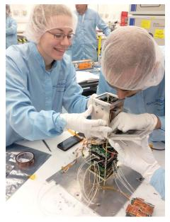
STRaND-1 took just 3 months to build and uses a Google Nexus One smartphone with an Android operating system. (Courtesy: AMSAT-UK)
