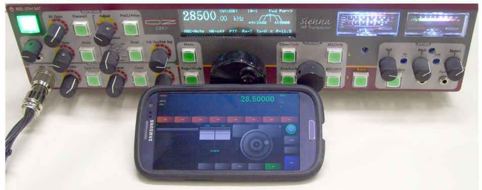
Sienna with Pocket Transceiver app running on a Samsung Galaxy SIII. The "cell phone" is connected to HRD's server via Wi-Fi. The HRD server is running on a PC that is connected to the rig (in this case a DZKit Sienna) via an RS-232 port.
