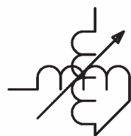
Fig 4 Variocoupler schematic symbol
