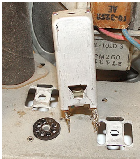
One of the "donor" transformers being removed from its chassis cutout in the junker clock radio.
