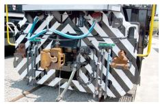
The event also provided an opportunity to get a close-up look at the new locomotives. Here, the rear of one of these new units has the EP (electro-pneumatic) braking equipment mounted just to the right of the coupler. rates
