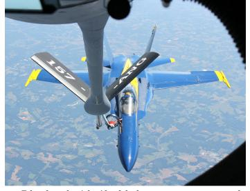
Taken from the right side of the boom operator, you can see the 'catcher's mitt.' It's hard to see but there is a flexible hose between the basket and the solid, straight boom. I chose the right position for this shot. People that were on the left side of the boom operator had a different angle; the tanker's boom blocks the cockpit. (Shutter speed 1/200 at f10 aperture)
