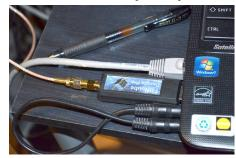
The FUNcubeDongle, often called a FCD for short, sets up when plugged into a PC USB port. In order to program the FCD, a free application is available from the folks in the UKat http://www.funcubedongle. com/?page\_id=313.
