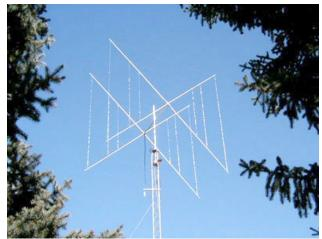
Two-band Cubex MKII cubical quad antenna. (Courtesy: Cubex Quad Antennas)
