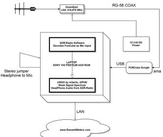
ates in the 217 MHz range and loaded the SDR-Radio and Argo software. The latest version of Argo supports FTP (File Transport Protocol). It allows you to send the latest image to a remote FTP server while Argo continues to log. The logs can be saved to any accessible location. I save mine to a high capacity 3 terabyte external network hard drive. Each file can be in the order of 85 to 110 kilobytes and the recordings happen about once a minute. Though this creates a lot of
