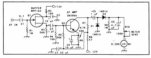
**Figure 1:** Schematic diagram of the audio-derived S meter. Capacitors are in uF. Polarized capacitors are electrolytic or tantalum. Fixed-value resistors are 1/4 watt. R10 is a PC mount carbon composition trimmer control. Q1 can also be a 2N4416 or other N-channel JFET. Q2 can be a 2N2222, 2N4400 or similar device.
