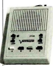
Ventriloquist requires 9 to 16 volts DC at less than 80 Ma. 60 mW of audio output is available to drive the internal speaker or an external device.
