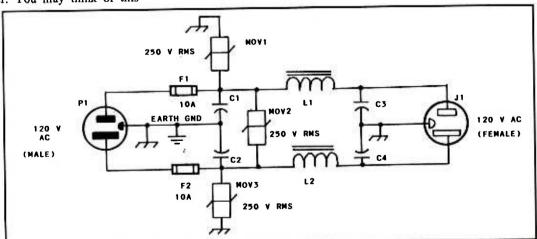
Figure 1: Schematic diagram of the line filter and transient suppressor. C1-C4, incl. are 0.01-uF, 1000-V disc ceramic (see text). F1 and F2 are 10-A fuses in standard fuse holders. 10-A circuit breakers may be substituted. L1 and L2 are 16-uH toroid coils (see text). MOV1-MOV3, incl. are described in the text. P1 is a male chassis-mount, three terminal ac plug. J1 is a female three-terminal, chassis-mount AC socket.
