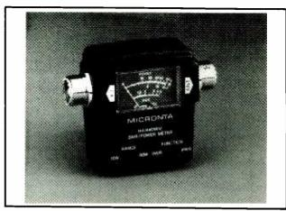
Figure 1: VHF/UHF SWR - Power Meter
