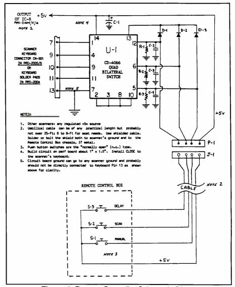
Figure 1: Remote Controller Schematic Diagram
