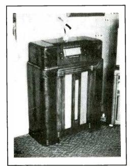
If your taste runs to large objects and you have an appreciation for fine woodwork, a console may be just the thing for you. This 1941 Silvertone model 7048 has some very nice mahogany on it. The radio has eight tubes and covers AM BCB and 6-18 MHz shortwave, including two bandspread sections for 31 and 25 meters.
