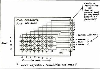
Figure 2: PRO-2004/5/6 Keyboard Switch Matrix Diagram
