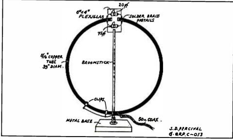
Figure 2 - G3BGR Loop Antenna
