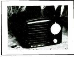
The other end of the spectrum, another Silvertone, but a baby brother to the console. This little fellow was made about 1947, tunes BCB AM only, and has four tubes. This AC-DC model has a resistance cord, and surprisingly good audio reproduction for its small size. The case is Bakelite. You don't need a garage to enjoy this hobby.
