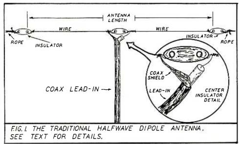
To determine the antenna's total length, in feet, use the formula L = 468/frequency in MHz.
