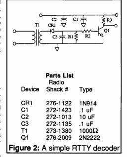
The transistor in Figure 2 provides the same amplification as the tube, except in this case the transistor drives the RS232.
