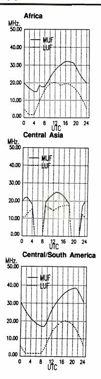
Once you've located the correct charts, look along the horizontal axis of the graph for the time that you are listening. The top line of the graph shows the Maximum Usable Frequency (MUF) and the lower line the Lowest Usable Frequency (LUF) as indicated on the vertical axis of the graph. The strongest signals will be near the MUF.
