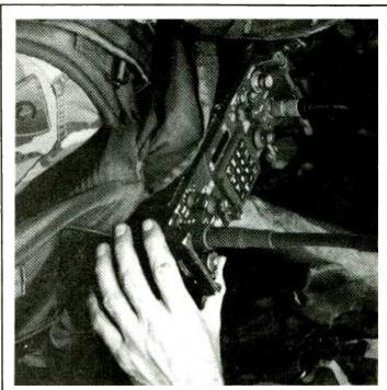
Desert Storm communications above 30 MHz were heard almost worldwide from these manpack radios, due to skip conditions. Disturbingly, much of it was in the clear.
