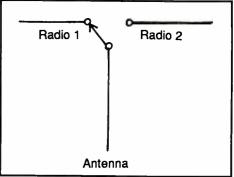
Simple SPDT switch configuration
