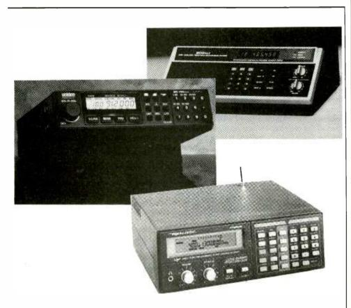
could well be the best scanner ever made. Its 400 memory channels are enough for just about anyone; user-selectable AM, FM wide and FM narrow modes provide additional -and useful - functionality. Frequency coverage of 25-520 and 760-1300 MHz (cellular excluded; easily restored) meets most anyone's needs.
