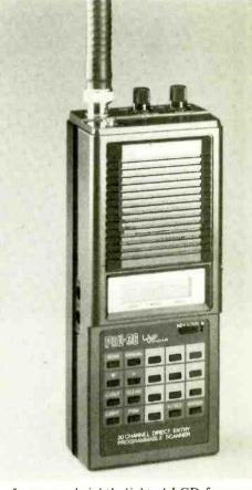
features a brightly-lighted LCD frequency display which is readable to 4 decimal places.
