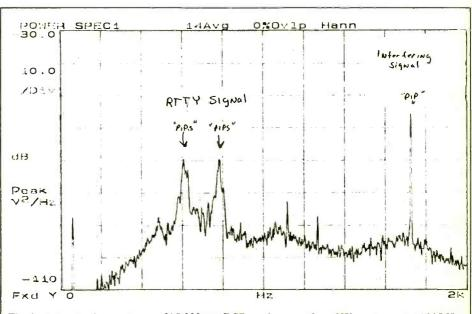
Fig. 2 - Actual printout from a \$25,000 HP DSP analyzer and an SW receiver at 16.907 Hz.
