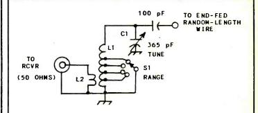
Figure 3 -- Circuit for a simple antenna tuner that is suitable for use with end-fed antennas of random length. See the text for construction details.
