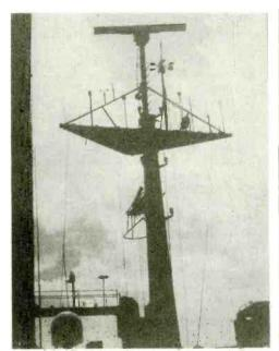
Ship's mast with communications and radar antennas.
