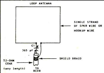
Figure 2 -- A small wire loop may be clipped to the wall and used as shown here. C1 is adjusted for peak signal response. The size of the loop is not critical. The larger the loop the better the performance.
