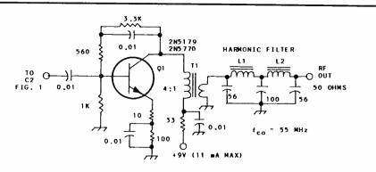
**Figure 2 -** Schematic diagram of a Class A RF amplifier for use with U1 of Figure 1. Decimal-value capacitors are in  $\mu$ F. Others are in pF. Capacitors are disc ceramic. Resistors are 1/4-W carbon.
