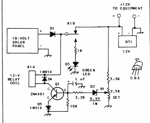
**Figure 2** -- Circuit for a solar panel with regulator circuit. The operation is explained in the text. D1 is a 100-V, 3-A rectifier diode. D2 is a 6.9-V, 400-mW or 1-W Zener diode. Fixed-value resistors are 1/4 or 1/2-W carbon film. R1 is a linear-taper carbon composition control. K1 is a low current 12V dc relay. It is shown in the normally open position (not energized). The 18-V solar panel has 36 cells wired in series.
