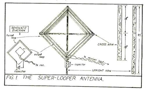
8. Insert the bottom end of the upright frame piece into the base, and attach the connector to your receiver. You are now ready to begin using this antenna.
