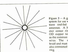
Figure 3 -- A ground-radial system for use with quarterwave end-fed or vertical antennas. A 10-inch diameter center ring (1/4-inch OD copper tubing) serves as the common point for the wires. The coax shield braid and mast or tower are also connected to the center
