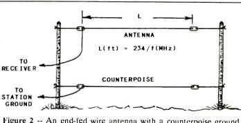
Figure 2 -- An end-fed wire antenna with a counterpoise ground below it. The counterpoise should be the same length as the antenna. The wire gauge for the counterpoise is not critical.
