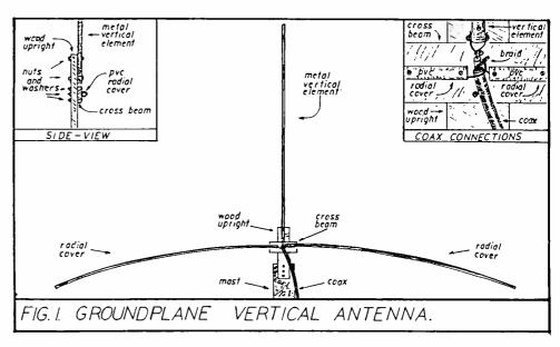
6. If you want a ten-meter antenna, cut the metal pipe (vertical element) to 8 feet 1 inch. Otherwise use the formula: length = 234/frequency. Here length is in feet and frequency is in megahertz (use 71.3/frequency if you want your length measured in meters).
