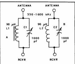
Figure 2 -- Toroidal (A) and solenoidal, air core (B) trap coils. C1 and C2 are ARCO no. 4611 mica compression trimmers for use from 550 to 900 kHz (300-1000 pF). For operation from 800 to 1600 kHz use an ARCO no. 466 (105 - 480 pF) trimmer. L1 has 35 turns of no. 26 enam. wire on an Amidon Assoc. FT-82-61 ferrite core. L2 contains 52 turns of no. 20 enam. wire, close wound on a two inch OD coil form that is three inches long.
