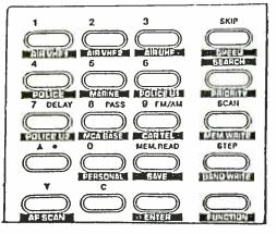
control all of the functions and is as much a computer as it is a radio. Because of this, the operation and programming of this unit is not quite the same as we have become used to with such radios as the Bearcats and Radio Shacks. You can't simply punch in a frequency and then hit ENTER to save the frequency in a memory channel. Most operations require two or more steps and are thus a bit more time consuming than with other hand helds.
