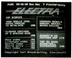
Electra Teletext via VBI on TBS Superstation G1,18. Produced by Taft Broadcasting of Cincinnati and received on Zenith TVs with built-in World System Teletext decoders.
