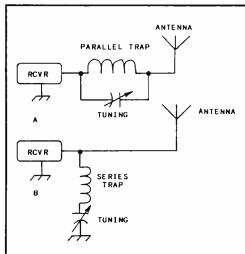
**Figure 1** — Examples of tuned traps. A parallel-tuned trap is shown at A. Example B is a series-tuned trap. Use the configuration that provides the greatest attenuation of the unwanted signal.
