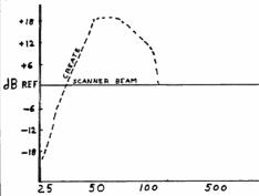
As seen from the accompanying graph, the Create was superior between about 49 and 110 MHz and the Grove was better below about 35 MHz. This was predictable since the Create is a true log periodic design with a sharp rolloff below 50 MHz, while the Grove is a hybrid log periodic with parasitic elements to enhance certain frequency ranges and one omnidirectional low band element at the rear.
