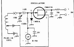
Figure 1 -- Schematic diagram of a functional gate-dip oscillator. The microampere meter reads the change in FET base current as the dipper is tuned to the frequency of the resonant circuit under test. Plug-in coils provide a wide range of test frequencies.
