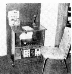
Fooled 'ya; inside the microwave/IV cart is a complete HF rig, 150 watts on 80 through 10. Sure does keep peace in the family when there is not enough room for a ham shack.
