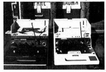
Motorola "Apcors," high power (12 watts) left, low power (1 watt) right
