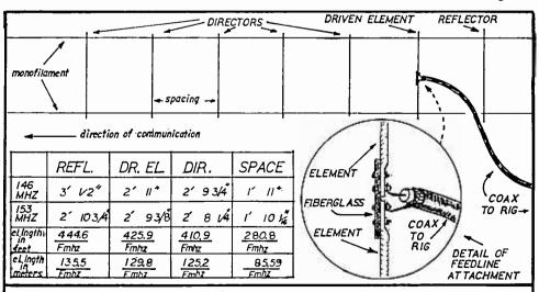
FIG.I. A 7-ELEMENT YAGI-UDA ANTENNA CAPABLE OF 12,7 DB; GAIN. THE TABLE GIVES ELEMENT LENGTHS AND SPACING.
