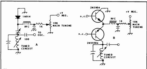
**Figure 1** -- The circuit at A shows how a common 1N914 diode can be used as a tuning diode. The capacitance change for a 1N914 is small. Two or more of these diodes may be used in parallel to increase the total capacitance. NPN transistors are used as tuning diodes at B.
