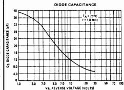
Figure 2 -- A characteristic curve for a Motorola MV209 tuning diode. Note the nonlinearity of the capacitance change versus operating voltage. This illustration courtesy of Motorola, Inc.
