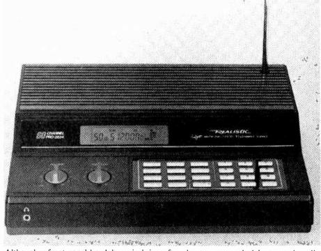
Although a front-panel headphone jack is provided, anti-blast protection built into the scanner reduces the audio substantially when an external speaker is connected to that port.
