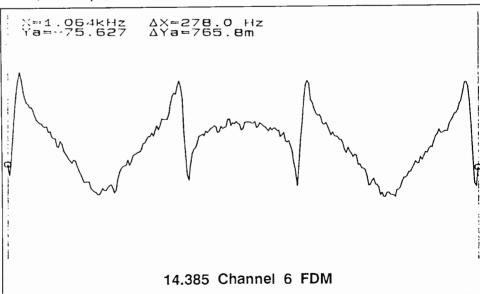
IS IT BATMAN? No! This is what a single channel of an FDM (Frequency Division Multiplex) RTTY signal looks like on a \$25,000 Hewlett Packard audio spectrum analyzer using a Sony ICR2010 on 14.385 MHz.
