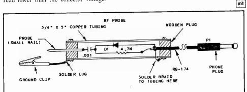
Figure 2 -- Circuit and physical details for an RF probe. D1 is a 1N34A or 1N60A germanium diode. A similar probe may be constructed for DC voltage measurement. Simply eliminate the inner capacitor, diode, and resistor and make a straight-through connection to the probe tip. See text for additional information about this RF probe.
