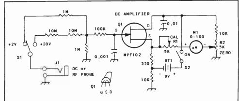
**Figure 1** -- Schematic diagram of the RF/DC meter. Capacitance is in uf. K=1000. M= million. BT1 is a 9-V transistor-radio battery. S1 and S2 are mini toggle or slide switches. R1 and R2 may be PC-mount trimmer controls (see text). You may use any 100-uA meter for M1.
