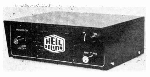
For \$450 the Heil SC-One! comes to the rescue of the avid SCPC listener. The SC-One! measures 9-1/2"x7-1/2"x3" and includes cables and 950-1450 MHz splitter and program guide chart.
