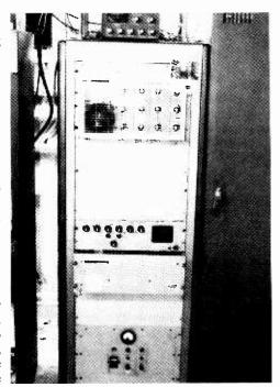
The high frequency transmitter used on the 4 MHz band by WJG-Memphis
