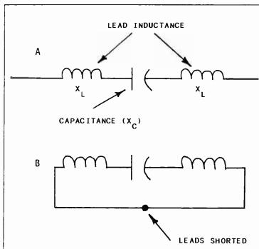
**Figure 1** -- Illustration A shows the effects of unwanted lead and internal inductance in a capacitor. In effect, we have a capacitor in series with two coils. The PC-board elements or other wiring associated with the installed capacitor add to the unwanted inductance  $(X_L)$ . Example B shows that if the capacitor leads are shorted together, we have a tuned circuit formed by the capacitor and the stray inductance (see text).
