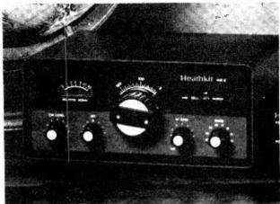
manual. Transmitter output power is about 2 watts.
