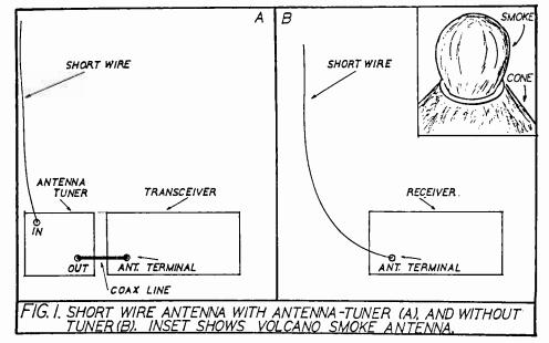
easier antennas to build. First decide what space you have available which is appropriate for mounting an antenna. Along the wall, on the ceiling, in the attic, and under the rug are places that have worked for many people.
