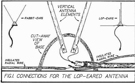
the coax out where you can work with it, trim its insulation back to expose about one inch or so of the inner conductor wire. Check the wire and make sure it is clean, as discussed above. Then twist the end of the inner conductor wire together with both the exposed ends of the short piece of twinlead cable wire you prepared earlier. Be sure to leave enough slack in the wires attached to the elements so that the elements can be moved on their pivots without breaking the wires.
