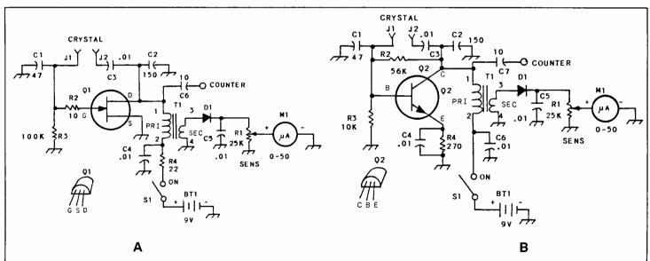
Fig 1 - Schematic diagrams of two crystal testers.
