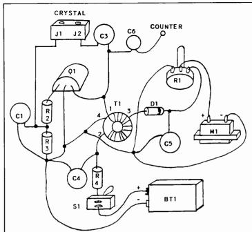
Fig. 2 -- Pictorial diagram of the circuit in Fig. 1A. This shows how the parts are connected together. Keep in mind that the component leads (except for the dc leads) must be kept much shorter than they are depicted here.
