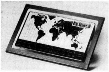
A similar unit from Seiko, the World Time Touch Sensor, allows you to touch any city or time zone on the world map covering the face of the unit, and the clock instantly displays time, day and date. Time can be digitally displayed on a 12 or 24-hour basis, with a daylight saving time button and 27 different time zones. Suggested retail is \$95.
