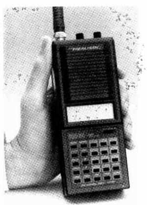
plastic case and features a two-tone colorcoded keypad. A grey background is used behind the scanner's function keys with blue designating the digits 1 thru 0. A top-lit LCD display is provided for frequency and function readouts and is one of the few which is readable in all lighting conditions, including complete darkness.
