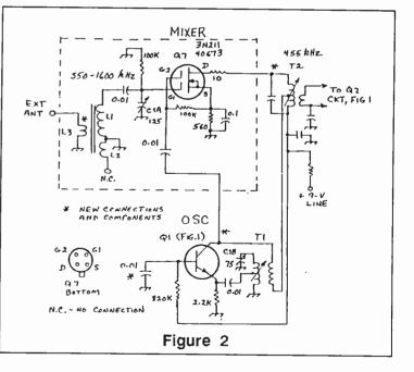
Fig. 2--Schematic diagram of the changes needed to improve the performance of a typical AM transistor radio. Q7 is a new transistor that is used as a mixer. Q1 has been altered to function only as an oscillator, rather than as a mixer/oscillator (see text). P-P oscillator voltage to G2 of Q7 should be 4 to 6 volts for proper performance. Increase the supply voltage to Q1 if the injection voltage to Q7 is low.
