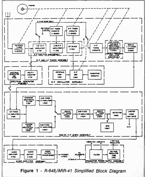
amplifiers until full receiver sensitivity is achieved. The other half of IV-506 is a noise limiter which suppresses undesired noise pulses.
