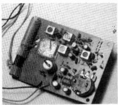
cutter bit also suitable) to form a grid of 3/16 inch isolated square pads. The transistor and components are soldered to these pads. The tiny module is mounted atop the radio PC board near the loop antenna.
