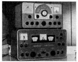
Photo 1: Ranger transmitter and HQ-170 receiver = CW/AM operation from 160 to 6 meters with 65 watts of power.
