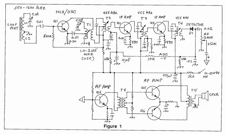
tunity to touch up the slugs in T2, T3 and T4 of Fig. 1. Adjust them for maximum audio output in the speaker while listening to a weak station.
