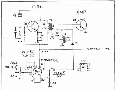
**Fig. 2** -- Schematic diagram that shows the changes to the Fig. 1 circuit for using voice or music transmissions. Q3 of Fig. 1 is eliminated. R1 is a linear or audio taper carbon control. U1 is a National Semiconductor Corp. Audio amplifier Ic, 8 pin DIP.
