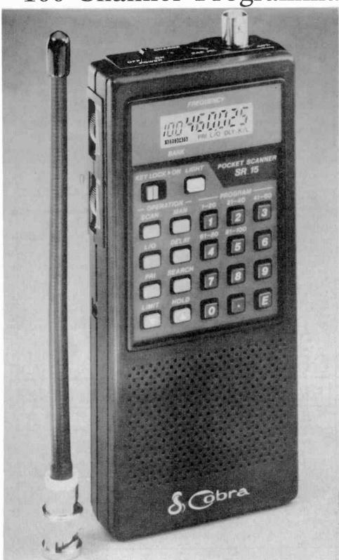
One of the newer additions to the evergrowing number of "mega-channel" handheld scanners if the Cobra model SR15. Measuring a scant 2-3/4"W x 6"H, and weighing only 10-1/4 ounces, this one truly meets the meaning of a "pocket scanner." Its small size, coupled with its 100 channel capability, make the SR 15 quite versatile.
