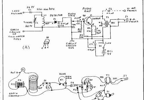
Fig. 1: Schematic diagram (A) of a simple diode-detector AM broadcast-band receiver. The resistors are 1/4 watt carbon composition types, except for R1, which is a potentiometer. The drawing at B shows the same circuit in pictorial form.
