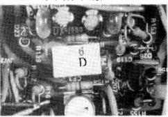
Typical Stock IF Filter installed in a Bearcat DX-1000
