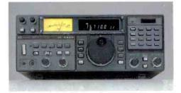
The IC-R71A is a shortwave listener's delight. Its 32 tunable memories store frequency and mode information, and they are single-button reprogrammable independent of VFO A or VFO B's operations! This HF reception is further enhanced by a dual width and level adjustable noise blanker, panel selectable RF preamp, selectable AGC, four scan modes, and all-mode squelch.
