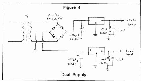
times raise the input voltage enough to get by at maximum load. Don't get carried away adding capacitance tho-- see next hint.
