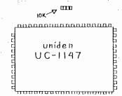
6. Using miniature wire cutters, cut the resistor body in two without disturbing
