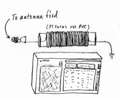
The signal from the Caribbean Beacon on 1610 kHz is boosted as the coil around the PVC pipe is brought nearer to the receiver's internal ferrite rod antenna.
