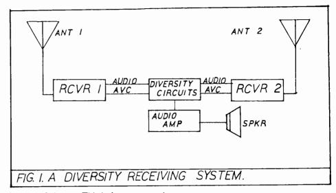
from one fades out. This isn't too easy and you may end up spending most of your time switching instead of listening. Another approach to the problem is to simply have two receivers, each connected to a separate antenna. Tune them to the same frequency and both play simultaneously.
