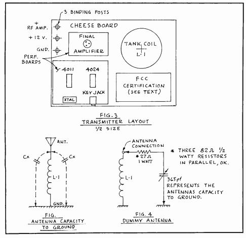
antenna. This will require a means for "fine tuning" the tank/antenna coil. Changes in weather and moving the operational frequency will require retuning. I use a ferrite rod that can be moved up or down within the coil field at the top and then clamped in the desired position. As the ferrite rod penetrates the coil field, it increases the coil's inductance. Another scheme is to use a variable capacitor connected between the antenna and ground.
