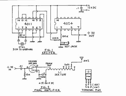
All resistors can be 1/4 watt. Capacitors should have a 50 volt minimum rating. A standard transistor socket can be used for the final amplifier.
