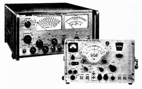
Popular among VLF listeners are commercial or military surplus frequency selective voltmeters like the Rycom R2174 and noise measuring test sets like the Ailtech NM17/27A and Singer NM25T shown here.
