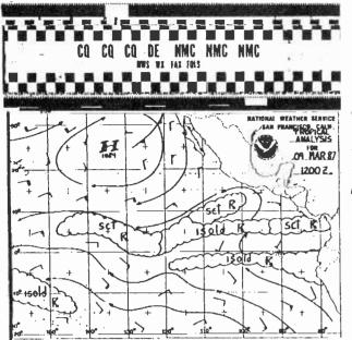
With an Epson graphics compatible printer, you can use the PK-232 in FAX mode to receive weather pictures or even wire-photos!
