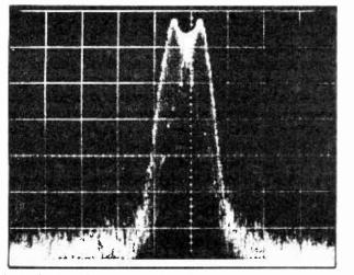
A single signal can be studied for modulation properties at minimum dispersion.
