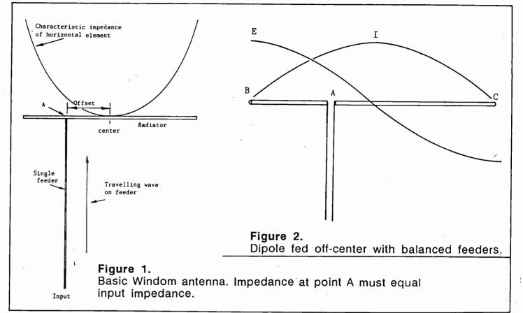
vertical radiator and the ground is its counterpoise; No precise method for locating the offset feed point which is a function of the input impedance of the vertical section. Published feed point locations vary from 0.037 to 0.083 wavelength from center.
