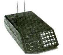
The new Regency TS-2 boasts the fastest scan and search rates in the industry—50 channels per second—more than three times faster that the next closest competitor. Six memory banks store up to 75 separate frequencies, selectable by groups or in a continuous sequence.
