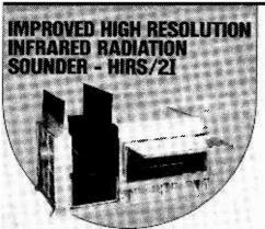
sea surface temperature. Data from channel four alone can be used as an infrared "window" to measure day and night cloud distribution as well as measure the temperature of the surface.
