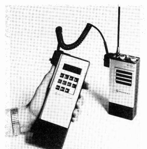
A special DVP code-inserter programs a specially-equipped (MX-series) hand-held for voice security (Courtesy of Motorola)
