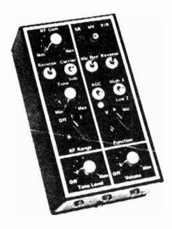
Bug detectors come in many forms: ACM-2 Countermeasures Instrument pictured above aids in the detection of hidden microphones, carrier current transmithidden tape recorders, concealed video cameras, telephone taps and bugs, telephone eavesdropping modifications, visible and infrared light attacks, and RF subcarriers. Easier for the novice to operate is the "Superhound" by Ross Engineering, pictured on the right.
