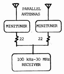
better match to the receiver is achieved if the outputs are isolated by two 22 ohm, 1/4 watt resistors as shown in the illustration.
