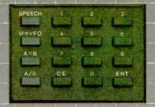
Keyboard Entry. ICOM introduces a unique feature to shortwave receivers, direct keyboard entry for simplified operation. Precise frequencies can be easily selected by pushing the digit keys in sequence of frequency. The frequency will be automatically entered without changing the main tuning control.
