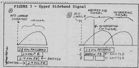
signal could be tuned in using the lower sideband mode (exalted carrier single sideband--ECSS). Since both sidebands of an AM signal carry identical information and the interference is affecting only the upper sideband, a good quality signal would likely result from this method.
