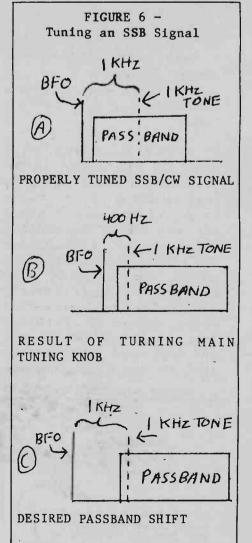
tuning knob has been turned, resulting in improper spacing between the signal and BFO. Our 1 kHz tone contained in the signal will now sound like a 400 Hz tone. Any associated voice modulation would likely be unintelligible.
