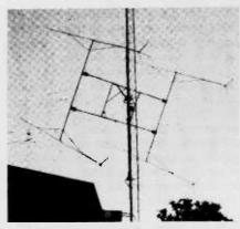
Fig. 4—K7KOT has incorporated his EME array into his existing antenna system by side mounting it on a tower.
