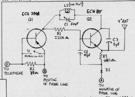
Schematic diagram of FM phone transmitter. D1 rectifies the AC current during the ringing cycle.
