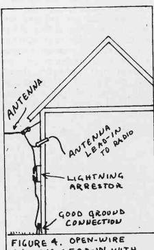
ANTENNA LEAD-IN WITH SPARK-GAP TYPE LIGHTNING ARRESTOR
