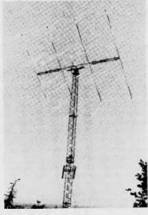
Fig. 3-This 2-meter EME array at I2ODI is built from 16 long-boom Yagis. Arrays like this are great to have, but smaller antennas can
