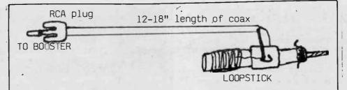
Figure 2-If you have an AM radio w/o external antenna terminals use this coupling setup. Position loopstick alongside radio's internal ferrite bar antenna--vary position slightly until best reception is achieved.
