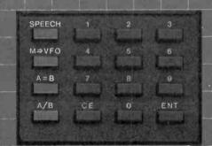
Keyboard Entry. ICOM introduces a unique ferture shortwave receivers...dirett keyboard entry for simplified operation. Precise frequencies can be easily selected by pushing the digit keys in sequence of frequency. The frequency will be automatically entered without changing the main tuning control
