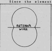
Fig. 2. The horizontal radiation pattern of a horizontally mounted dipole antenna. Note that the antenna has some directionality, as the gain, or response, of the antenna is maximum for signals that are perpendicular to the length of the antenna, and minimum (null) for signals off the ends of the antenna. If the dipole antenna is mounted vertically, as in figure 1C, its horizontal radiation pattern is circular, and the antenna is non-directional.
