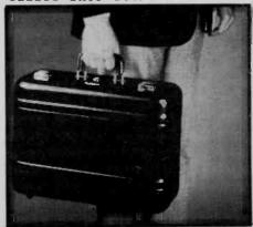
Motorola is recognized as a prime contractor for agencies of the federal government. Shown here is one of their new portable repeaters, capable of providing clear or encrypted speech in the 136-174 MHz (or 406-512 MHz on other models) running 1.7 or 20 watts.
