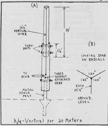
coaxial line back to the radial room is attached to the top bolt; the braid of the line to the bottom terminal.
