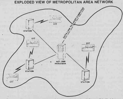
For metropolitan area coverage, a series of data transmitter/receiver stations are linked by tele-phone lines to a Network Control Processor (NCP-2000). This processor provides message coor-dination across the entire radio system, tracking location of the users, directing messages between the central computer and the user, and controlling the operation of the radio equipment.
